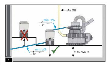
14. Connection of the amalgam separator ECO II with the EXCOM hybrid 1:
